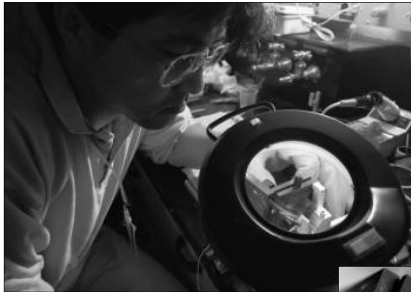
Los Alamos postdoctoral researcher Byoung Jin Suh assembles the force detector. The inset shows a closeup of the piezo electric positioner, the optical fiber and the cantilever.
