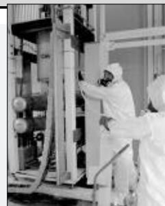
Employees from Advanced Nuclear Technology (NIS-6) perform a fuel exchange operation on the SHEBA assembly. The protective equipment, including respirators, is worn to guard against inadvertent contamination. Photo courtesy of
