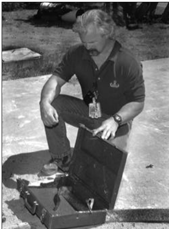
Brad Lounsbury of Emergency Management and Response (S-8) and leader of the Hazardous Device Team displays what's left of a briefcase shortly after being subjected to a mini-disruptor. The mini-disruptor made a small hole in the briefcase's side at the point of entry and blew out the side at the other end, which is exactly what should have happened. Photo by Fred Rick
