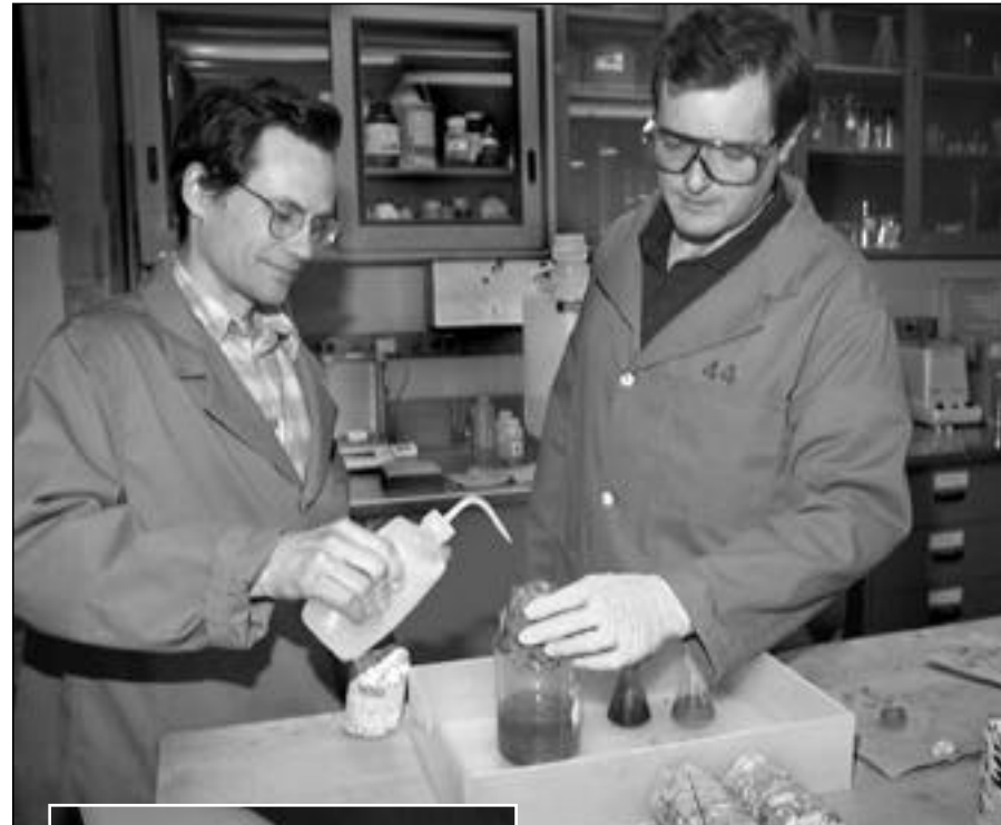
Bill Carey, left, rinses chemicals off a concrete core held by George Guthrie, before examining the core for the presence of alkali-silica reaction. Inset: An eyedropper is used to apply stain to a concrete core. The darker areas of the concrete core show where alkali-silica reaction has occurred. Photos by James E. Rickman
