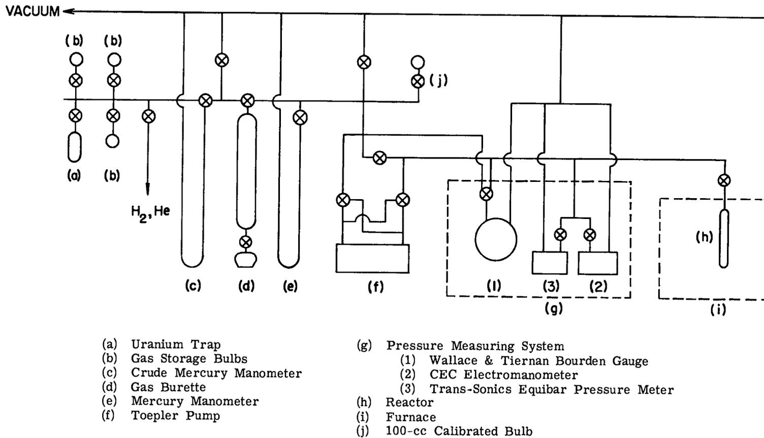
Fig. 1. Schematic of experimental system.
