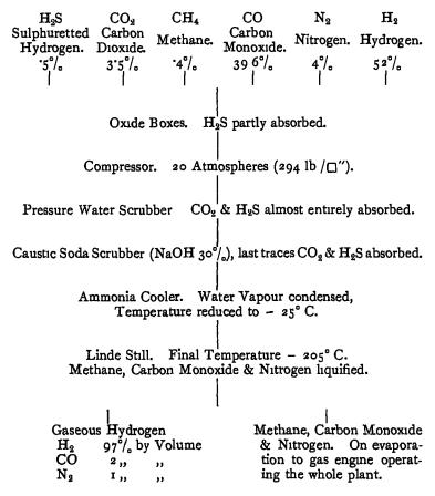
In the Linde-Frank-Caro process the blue water gas is compressed to 20 atmospheres, and under pressure it is passed through water, which removes practically the whole of the carbon dioxide and sulphuretted hydrogen. It is then passed through tubes containing caustic soda, which removes the remaining traces of carbon dioxide, sulphuretted hydrogen, and water.
