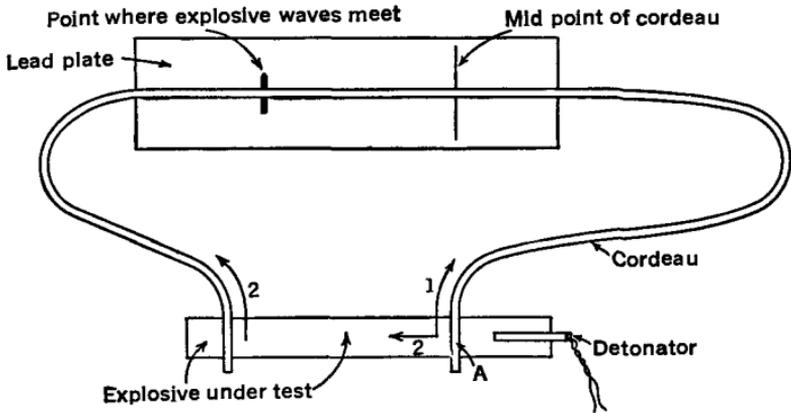
FIGURE 9. Dautriche Method of Measuring Velocity of Detonation. From the point *A* the explosion proceeds in two directions: (1) along the cordeau (of known velocity of detonation), and (2) through the cartridge of explosive which is being tested and then along the cordeau. When the two waves in the cordeau meet, they make a mark in the lead plate upon which the cordeau is resting.
