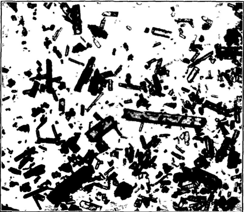
FIGURE 49. Commercial Sample of Ammonium Picrate (25×).
