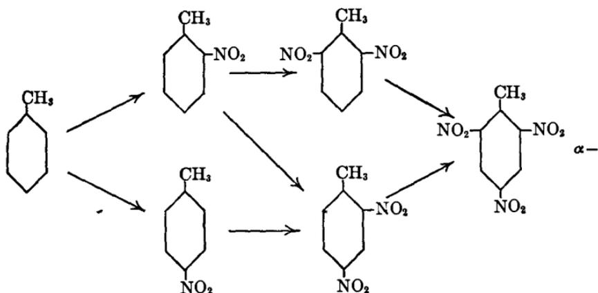
In industrial practice the nitration is commonly carried out in three stages, the spent acid from the trinitration being used for the next dinitration, the spent acid from this being used for the mononitration, and the spent acid from this either being fortified
