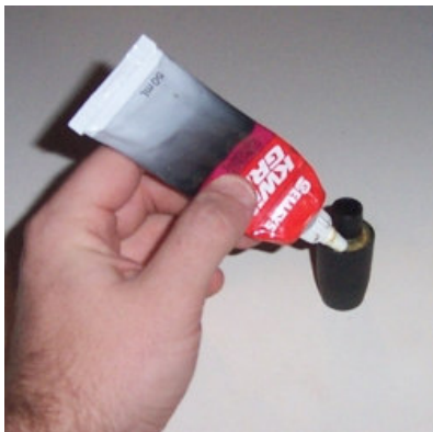
Figure 4 –adhesive is applied to upper notch in ball valve
