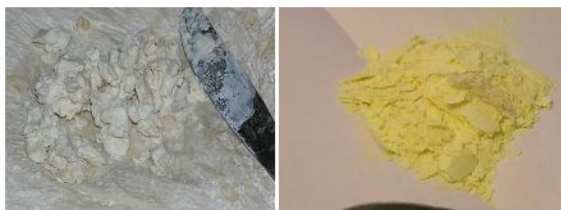
Figure 5: Drying crude precipitate (left); acetone extract of TEX (right).
