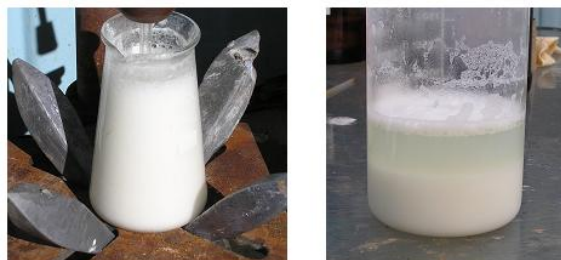
Figure 4: Nitration of DFTHP (left); fluffy precipitate in water (right).
