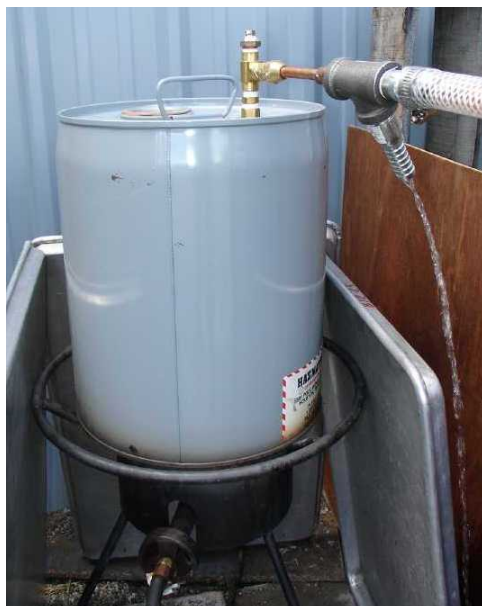
Figure 2: Ordenblitz's large-scale distillation apparatus
