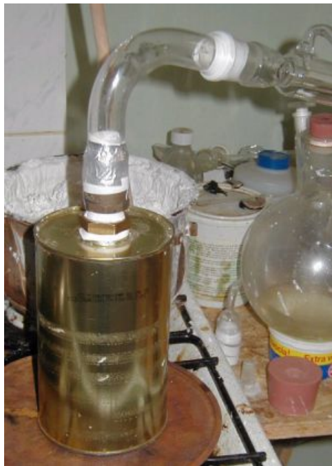
Figure 1: Robust metal can distillation apparatus
