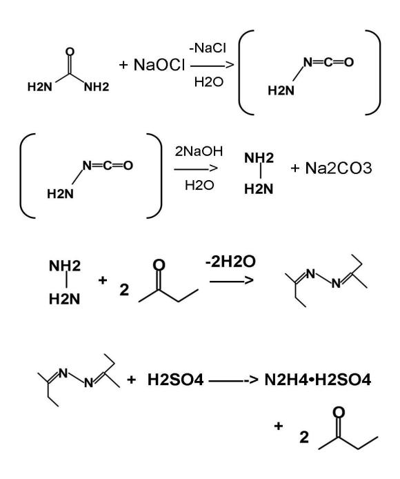
314g of 12.5% Sodium Hypochlorite (NaClO) solution was added to an Erlenmeyer flask and was chilled in an ice bath atop a magnetic stirrer. A stir bar was added and medium-speed stirring was begun.
