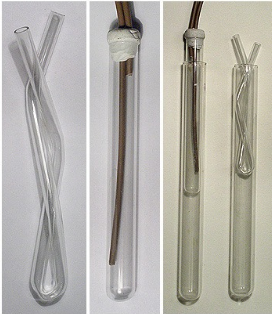
Figure 1: improvised condenser designs
