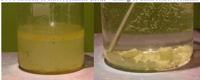
Figure 9: Nitration of chlorobenzene (left); washing of dinitrochlorobenzene (right)
