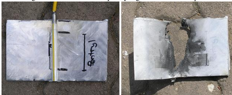
Figure 16: Detonation of pentryl against aluminium plate
