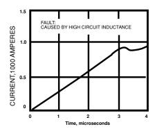
Figure 7 Marginal Firing Parameters due to Firing Set and Transmission Cable not Matched with EBW Detonator
