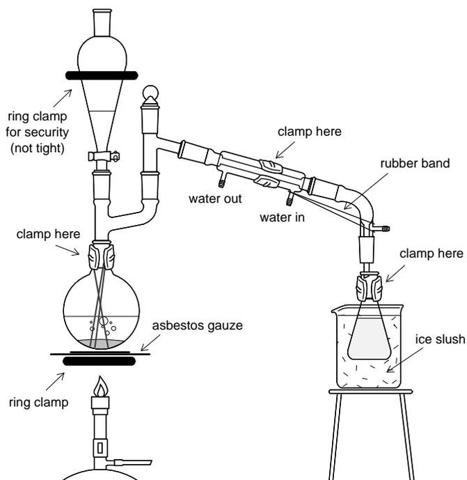
Mount the receiving flask onto a stand using a utility clamp. Use a tripod or a large ring clamp and wire gauze to position the ice-water bath. Use a steam-bath bowl or 1000-mL beaker for ice water.\* At least half of the receiving flask should be immersed in ice water.
