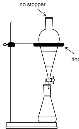
Transfer the dichloromethane solution to a 125-mL separatory funnel and add 30 mL of 5% potassium hydroxide solution. The solution is likely to warm up as the reaction generates heat.
