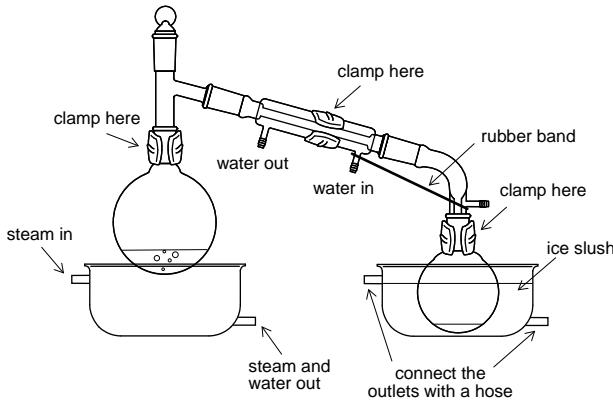
Distill off dichloromethane.<sup>†</sup> Do not heat too fast or foaming may become a problem. Stop the distillation when solvent no longer drips into the receiving flask.
