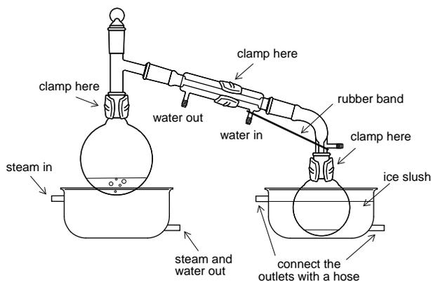
Distill off dichloromethane.† Do not heat too fast or foaming may become a problem. Stop the distillation when solvent no longer drips into the receiving flask.
