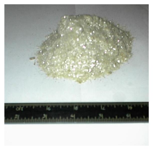
Same material (ETN) after protracted temp exposure. Product appears stable and maintains the same sensitivity. 3 - 5 mg when allowed a hammer fall (1.5 hammer) produced the same results. Seemingly no more or less.
