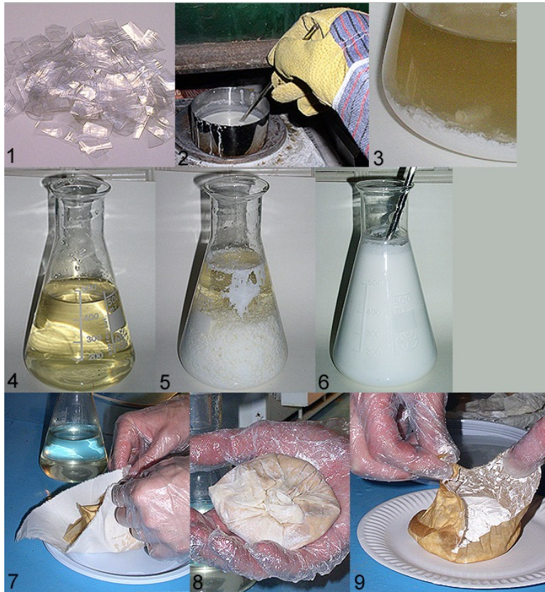
Figure 2: Illustrated steps of terephthalic acid recovery
