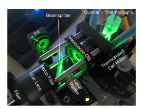
Figure 1 (supplement). Setup of the Raman spectrometer.
