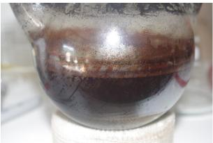
After a short time the purple became brown as the permanganate oxidizes the Xylenes and is in turn reduced to Manganese(IV) Oxide.
