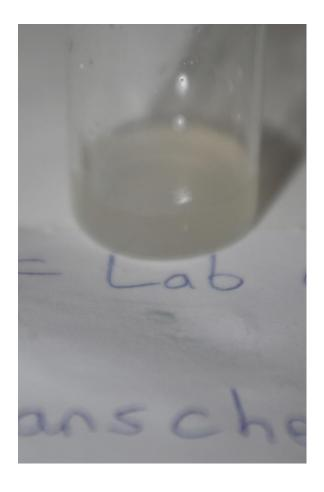
The mixture was left to separate for an hour and then the lower layer was drained into a vial for storage.
