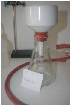
In the meantime a vacuum filtration system was set up, and the solution was filtered through a Buchner funnel to remove the insoluble gluten, starch and other binders. Alternatively, a gravity filter could be used, however is would be much slower.
