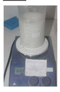
650mL of distilled water and 60g of 96% Sulphuric Acid were added to a 1000mL beaker and stirred until they were homogeneous. Be sure to add the acid to the water and not the other way around.
