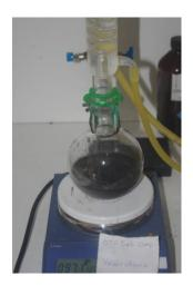
Low heat and reasonably strong stirring was switched on and the solution was refluxed for an hour. A second reflux condenser was placed on top of the first shortly after starting the reflux, as the smell of Ethanal could still be detected at the top of the first.
