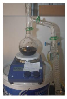
The mixture was heated to roughly 30C to boil off the Ethanal. Note that extremely cold condenser water is required for the reflux and the distillation to be able to condense the Ethanal.
