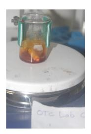
The heat was turned on and the Phenol and the Phthalic Anhydride melted. The stirring was then switched on and the solution began to go darker and darker orange. The Phenolphthalein is orange, not pink, because I used a little too much Sulphuric Acid, which caused the Phenolphthalein to be highly protonated into its orange form.
