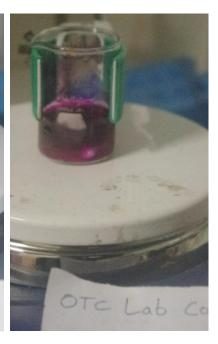
After an hour, the heat was turned off and 4g of Sodium Hydroxide in 20mL of water was added. The Sodium Hydroxide is acting here as an extraction reagent, nothing of it makes it into the product. The excess Sulphuric Acid is neutralised and the Phenolphthalein is deprotonated to its characteristic pink colour.
