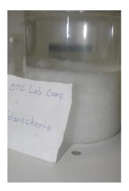
The mixture was refluxed for an hour and was then taken off heat and allowed to cool. The solution now smells strongly of Ethanoic Acid.
