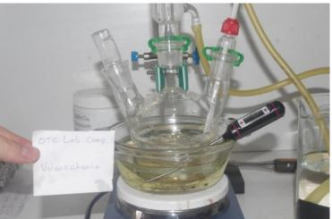
The hotplate was turned on and the oil bath was heated to approximately 85 degrees Celsius and maintained there for the remainder of the reaction. When the Xylene solution had reached 80 degrees, the stopper was removed and approximately one tenth of the Potassium Permanganate was added through the powder funnel. This resulted in an instant intensely purple solution.
