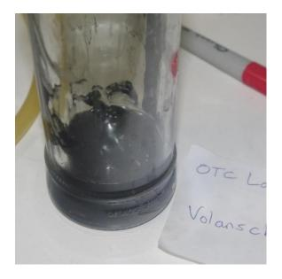
The Manganese(IV) Oxide in the filter funnel was washed with Ethanol to remove the Xylenes, and then water to remove the Ethanol and other soluble impurities. It was then placed in a jar where I dried it by heating it while under an airstream. This took a considerable amount of time.
