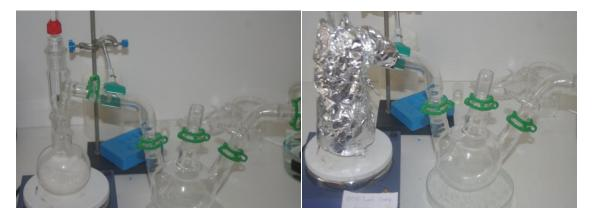
The heat was turned on and the 2-Hydroxybenzoic Acid first melted and then started to decompose. Some of the acid will sublimate onto the walls of the flask until the whole thing heats up enough to prevent this. The temperature was controlled so as to keep the still head temperature between 180C and 188C, so as to prevent distilling over impurities.
