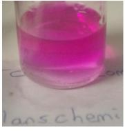
The solution was then poured into a small amount of dilute Sulphuric Acid, which neutralises the NaOH and crashes out the Phenolphthalein.
